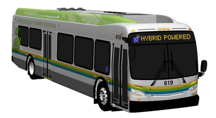
HEVs usually come with a technology called regenerative braking. This is a great feature that saves energy. Traditional vehicles completely depend on friction brakes to slow down, and in the process dispel a car's moving energy in the form of heat. Regenerative braking can harness some of that energy, which is converted into electricity and stored in the batteries for later use, such as running the motor or accelerating the car.
